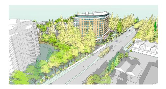
The curvilinear nature of the building form reflects the surrounding landscape and natural context. This form also relates well to the curves and orientation of the Roche Point Tower. A "fold" has been introduced along the curved north facing side of the building, which punctuates the main building entrance facing the parkway.
